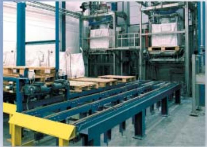
■ Big-Bag filling system for handling resin flakes
