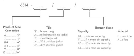
Example 1 6514-8-A/LC/1.2A Fireall gas burner complete with carbon steel jacketed tile and 1.2 capacity alloy nose
